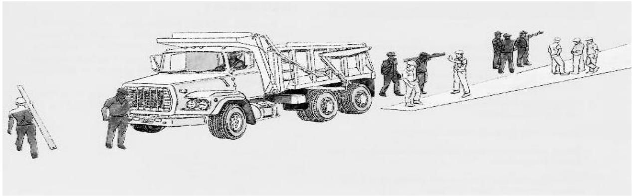
(Figure 4 – This illustration shows how some personnel on foot are visible to the driver while others are not. The driver cannot see the dark figure because they are passing through blind spots at the front and rear of the truck.)
