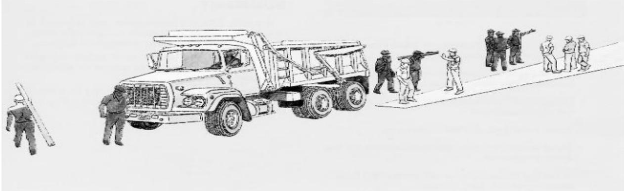
(Figure 4 – This illustration shows how some personnel on foot are visible to the driver while others are not. The driver cannot see the dark figure because they are passing through blind spots at the front and rear of the truck.)
